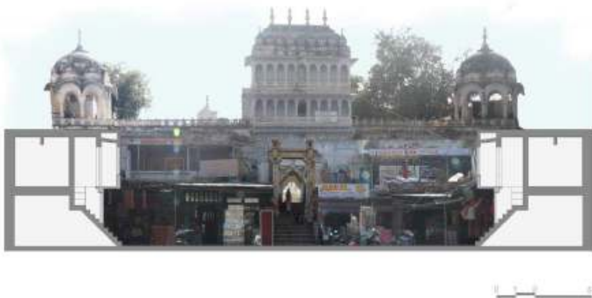
Figure 4: Section East-West of the Katla Bazaar, the old monastery converted into a new market area. The drawing shows the internal part of the structure which is also the old one (image by A. Fornaca, H. Joshi, M. Parmar, S. Caposciutti)
