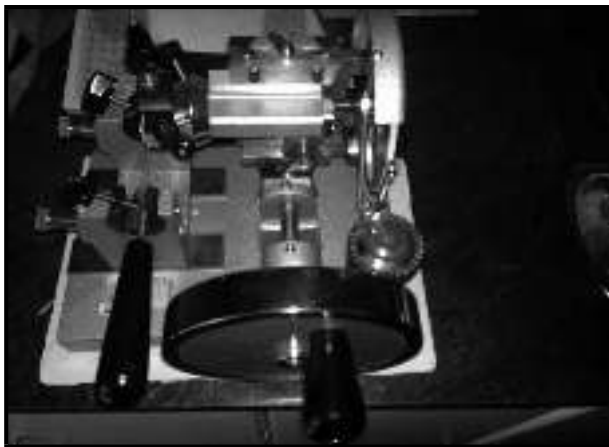
Figure 5: Microtome used to cut extremely thin slices
