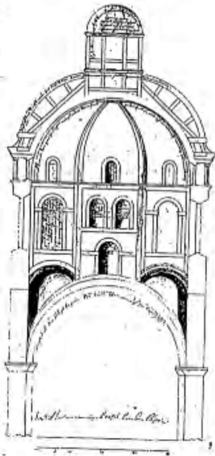
Fig. 5. : An early repair / strengthening drawing of the Dome of Fig. 4, [4], with enlarged windows.
