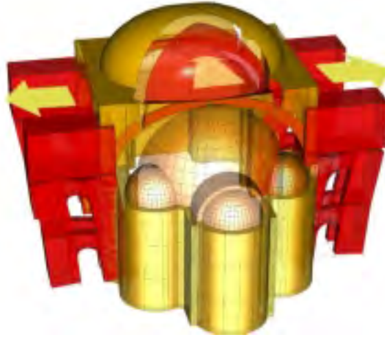
Figure 8. Collapse mechanism of the transversal main arches in the 10 th and 14 th century (drawing by L. Bianchini).
