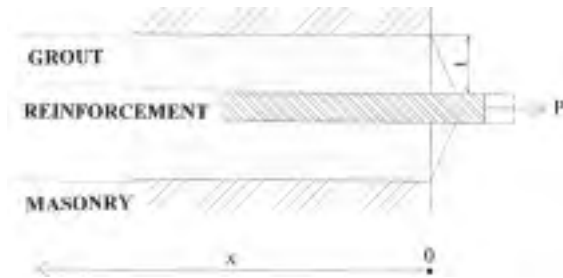
Fig. 1: Scheme of anchorage area
