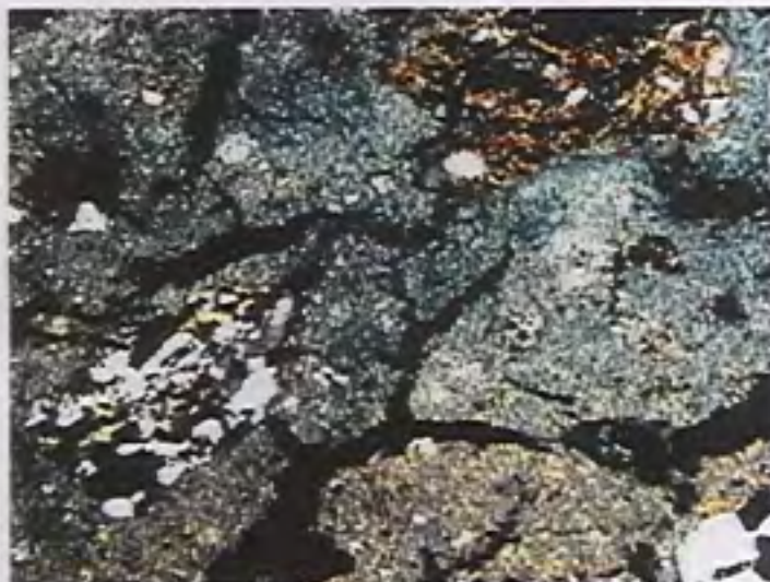
Fig. 2 Lime mortar structure of 5th century. Open cracks and large pores (x65)
