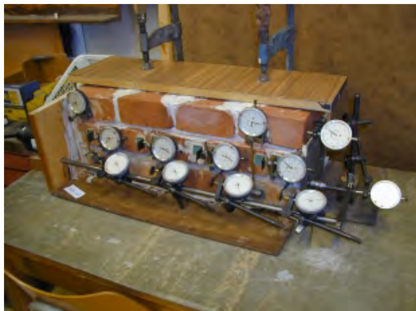
Fig. 7: Scheme of tests arrangement within the reinforcement anchorage in masonry
