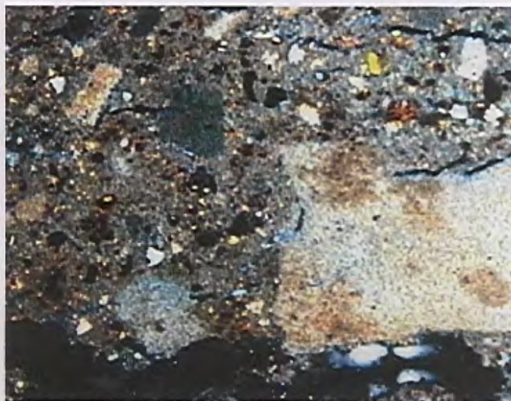
Fig. 3 Structure of pozzolanic mortar from 7 th century. Good cohesion between the crystal units (x65)
