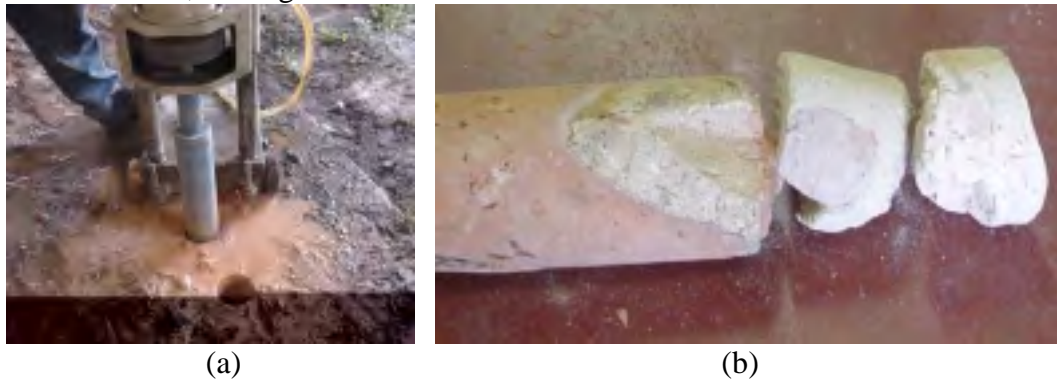
Figure 11 – Samples for mechanical testing: (a) coring and (b) sample
