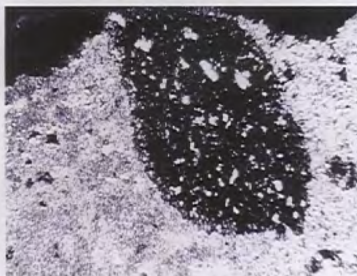
Fig. 6 Crushed brick as aggregate reacting with the binder and forming a reaction rim with thickness 50µm. (Galerius Palace, Polarized microscope x65)
