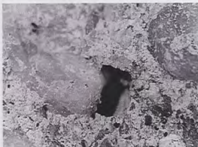
Fig. 9 Void in contact with an aggregate due to loose compaction (Stereoscope, x15)
