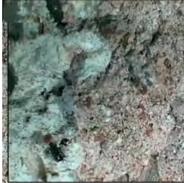
Figure 3. Cohesiveness between different layers of renderings (Stereoscope x10)
