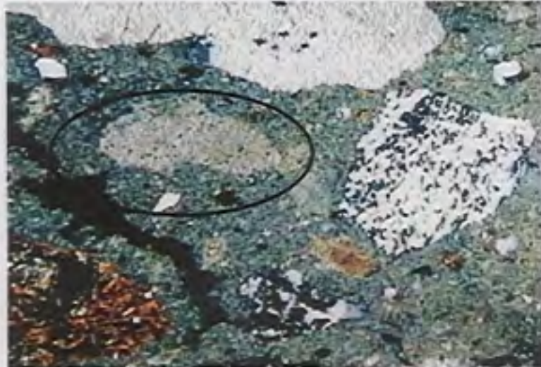
Fig. 1 Loose and dense structure in the binder (x65)
