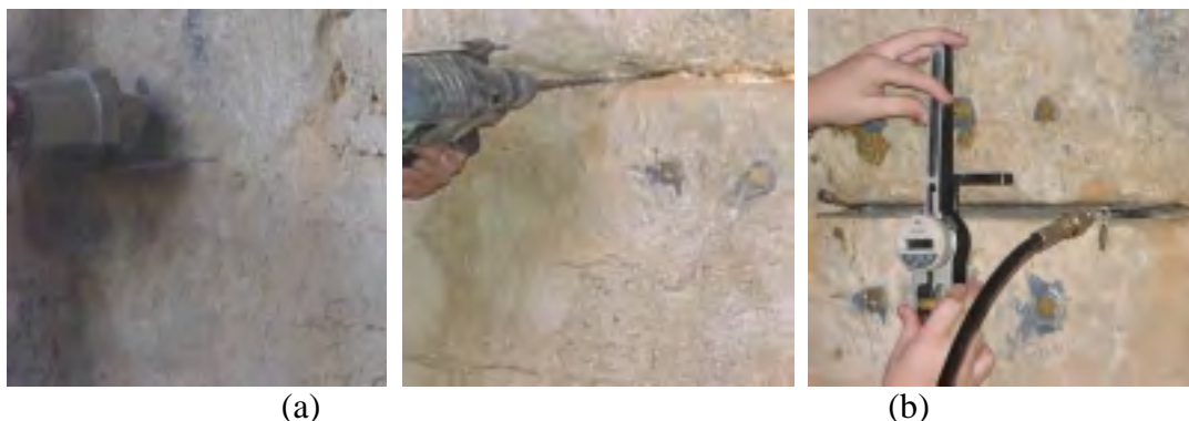
Figure 9 – Flat-jack testing: (a) Sawing the slot, (b) stitch-drilling the slot and (c) measuring operation
