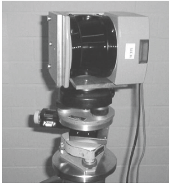
Figure 2: Photo of the 3dLMS laser scanner [6]
