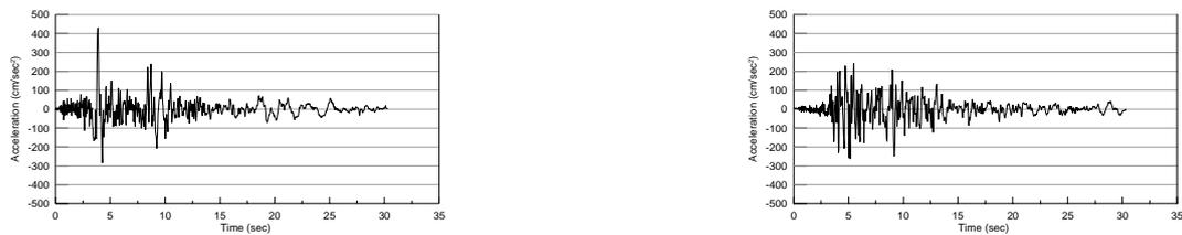
Figure 4: Horizontal components of the ground acceleration used in the analyses.
