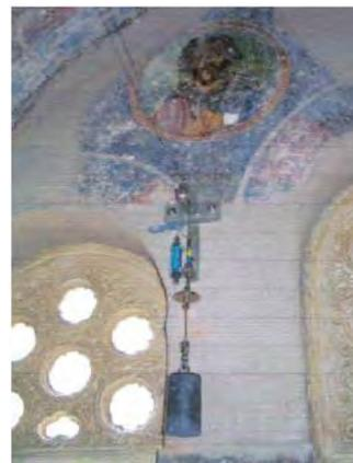
Figure 2: Displacement transducer, installed in the Katholikon of Hosios Loukas Monastery, Greece (photo A. Miltiadou)
