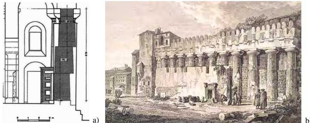
Figure 5. Detail of a damaged column (a) and view of the intervention following the earthquake in a picture of the XVIIIth century (b).
